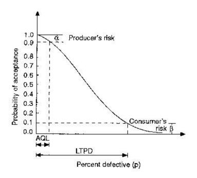
The concepts of the two types of risk are well explained using an operating characteristic- curve. This curve will provide a basis for selecting alternate sample plans. For a given value of sample size (n), acceptance number (C), the O.C. curve is shown in Fig..
